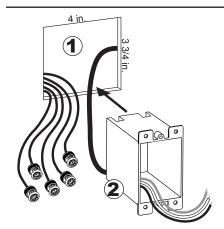
Select a location close to the head-end source equipment. Cut a 4-inch wide by 3 3/4-inch high hole in the wall. Feed the In-Wall power cable (not included) and signal-wires (not included) through this opening and route them to the location of the Power Outlet Faceplate.
